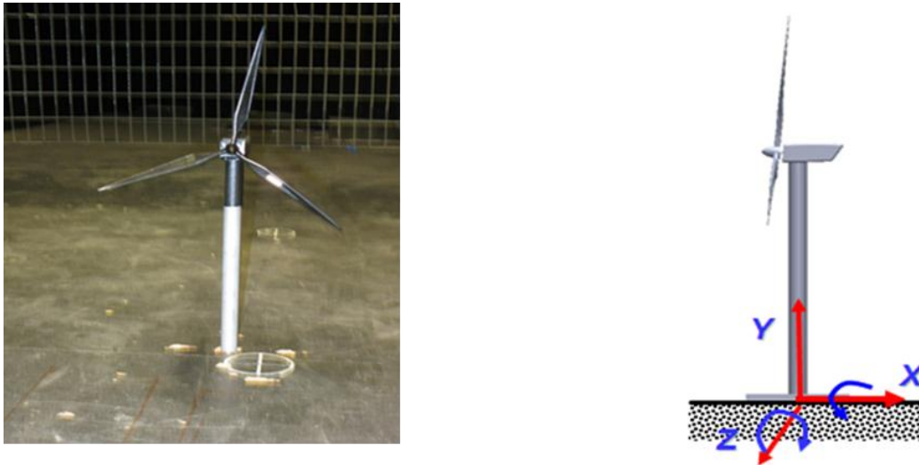
Figure 3-6 1:350 scaled wind turbine model to simulate a 2 MW wind turbine with 90 m rotor blades
