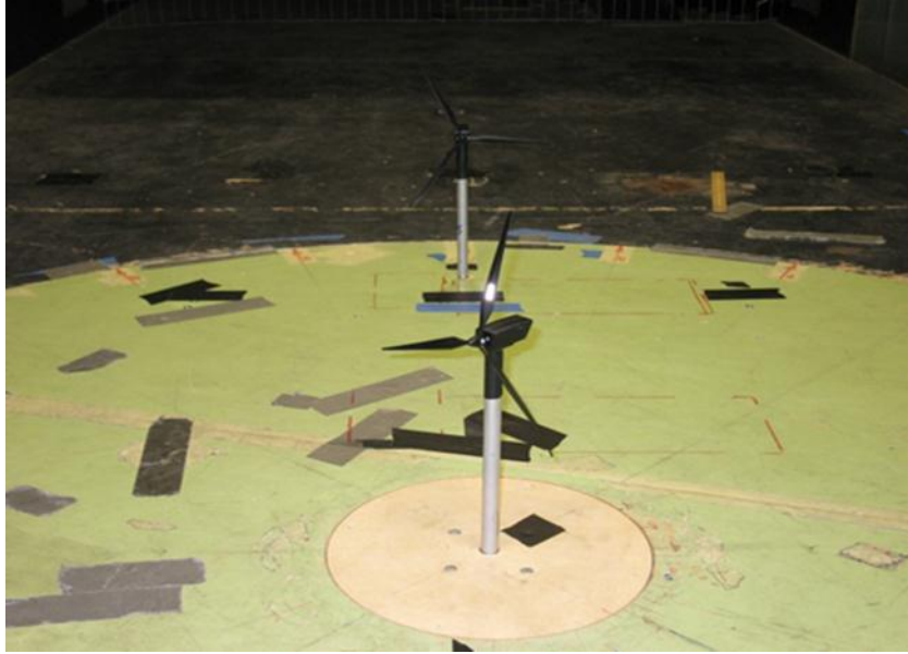
Figure 4-10 Two turbines in tandem arrangement with upstream turbine yawed with 50^\circ on the turntable
