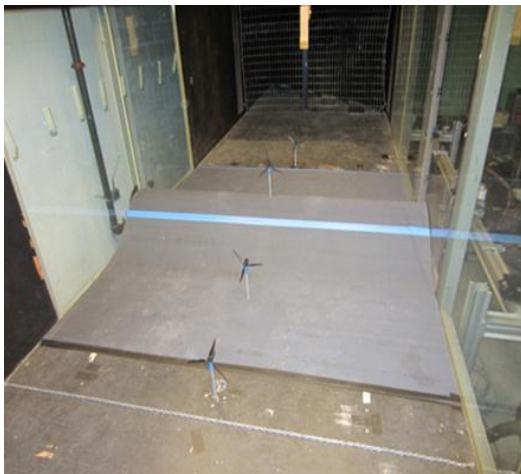
Figure 3-4 2D-Ridge profile with wind turbines installed around the ridge (left) and cobra probe measurement set-up on the top of the ridge (right)
