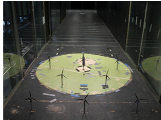
b) STAGGERED WIND FARM (3D)
