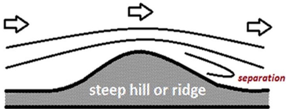
Figure 3-7 Schematic of the flow over steep hill or ridge, separation is likely to occur on the lee side depending on the slope
